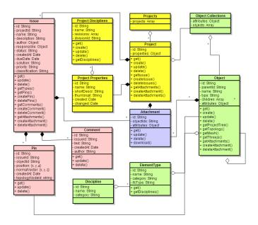
Fig. 1. Web API Object Model and Services diagram
